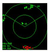
The Easy display consists of two concentric circles with a pie wedge. The circles are range rings and the pie wedge is the view your radar sees in front of you (the radar cone). You are located in the center of that circle and the view is a god's-eye view looking down.
